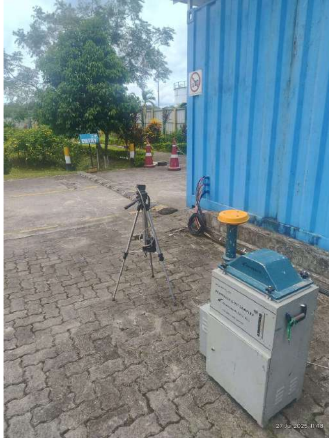
Ambient Air Quality Monitoring Near Security Main Gate
