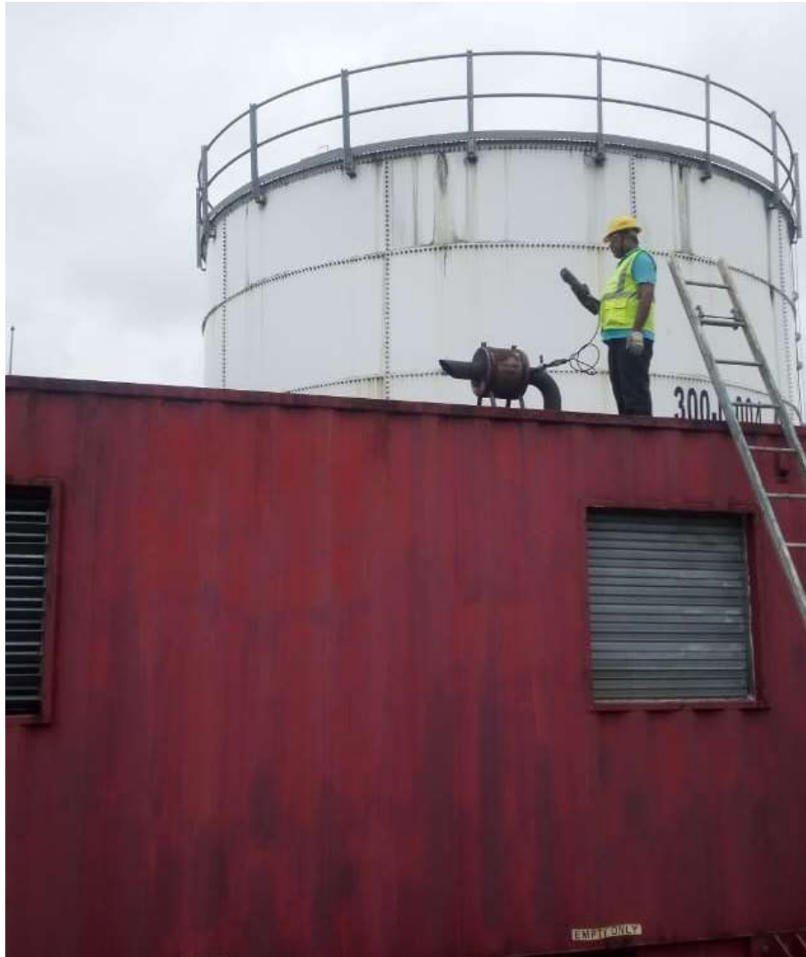
Flue Gas Monitoring Fire Engine No-2(B) Sl. No.: CD 6068B128481
